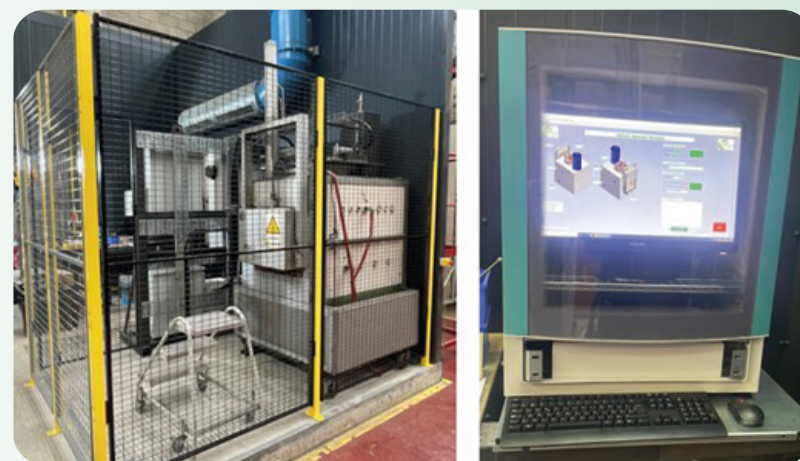
Laboratory hybrid reheating furnace for continuous monitoring of heating elements during operation
