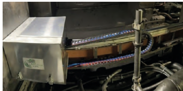
In-line sensor for measuring with high precision the Back-Up Roll (BUR) wear in a 6 high cold rolling mill
