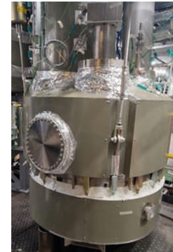
Vacuum pre-conditioning furnace for scrap de-zincing and de-coating
